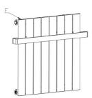
Finally, fit the radiator valves (not supplied) and connect to the pipework. Make sure that all joints are secure. Check that all fittings are fully tightened before filling with water.
