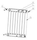
4. Fix the towel bar in the corresponding position on the product, then put the screws through the holes on towel bar and screw them into the sliding block (sliding block C placed in the middle of 2 vertical tubes in the appropriate position) on the front side, and then fix the towel bar on the product.
